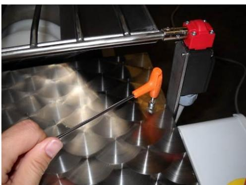
Extraordinary maintenance is particularly recommended at work end: disassemble the mesh cylinder as described below.
