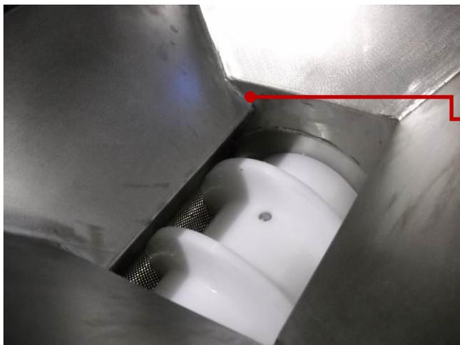
The special shape of the hopper, allows for a more even distribution of cappings inside the screw feeder, with no accumulation.
