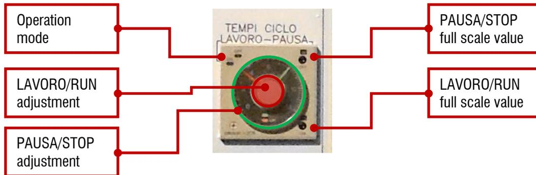
In addition to adjustment of the screw feeder rotation, it is also possible to easily manage run/stop cycles during rotation of the screw feeder.
