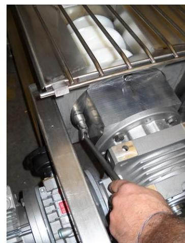
***CAUTION! Do not pull the cylindrical cage out, using iron hammers, levers or other tools which may damage the surface of the cage thus impairing proper screw feeder-cage coupling.***
