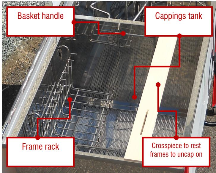
Rest the frame to uncap onto the wooden crosspiece.
