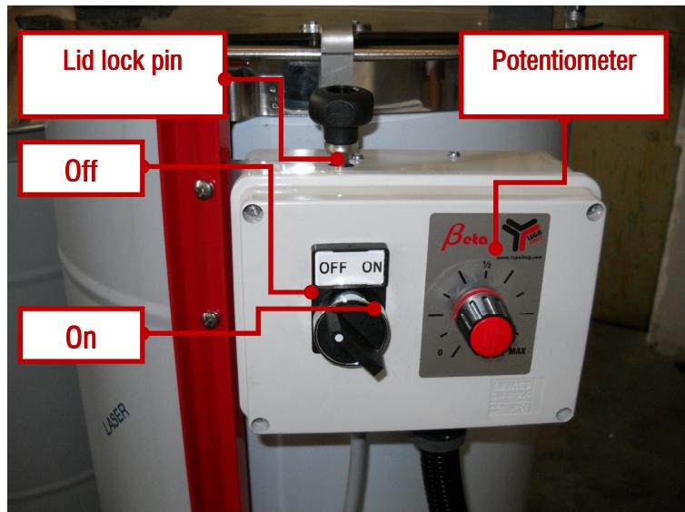
Arrange the frames evenly inside the cage; close the half-lid and turn the direction of rotation selector to the desired position.
