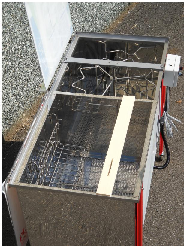
Clean the tank, the cage and all the parts that will be in contact with honey using a mild detergent. Then rinse with plenty of water.
